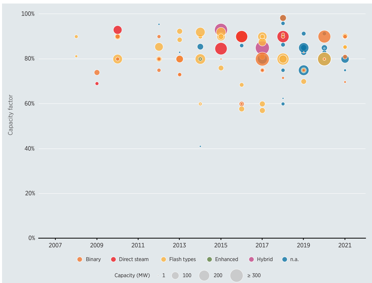
Figure 6.3 Capacity factors of geothermal power plants by technology and project size, 2007-2021
